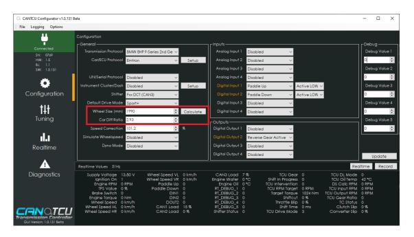
2. Drive the car and follow Realtime-values **TCU Output RPM** and **DS Calc RPM**. If you are unable to watch the values during driving, you can record a log and stop to check values afterwards.
